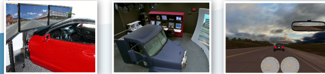
L to R: The NADS MiniSim system used as a base for a fully-mobile corvette simulator, the NADS-2 simulator (Freightliner cab loaded), an example of the visual system of the NADS MiniSim
